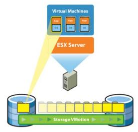
originating. This visibility allows storage and VM administrators to monitor for hot spots on the LUNs. When two or more VMs that are demanding higher IO than other VMs, they can be moved using VMware's Storage VMotion technology. Storage VMotion, as the name suggests, moves running VMs from one LUN (VMFS) to another without any downtime. VMs and applications keep reading and writing data without interruption or loss.
