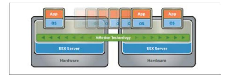
VMware vCenter monitors CPU and memory utilization of each VM on each server within a cluster. The Dynamic Resource Scheduler (VMware DRS) uses this data to automatically move VMs from a highly utilized server to a relatively less utilized server within the cluster. This keeps the hosts in the cluster load balanced.
