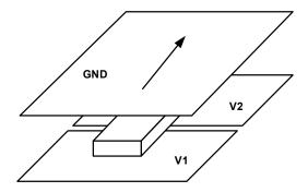
• When routing adjacent to only a power plane, do not cross splits.
