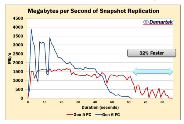
The replication process began with a massive copy request of all database objects defined in the replication parameters. Large block reads fed 1MB writes to the snapshot repository. The higher bandwidth of Gen 6 FC was leveraged by the snapshot process, resulting in completion of the entire process roughly thirty seconds sooner than with Gen 5 FC. That is nearly a third faster.
