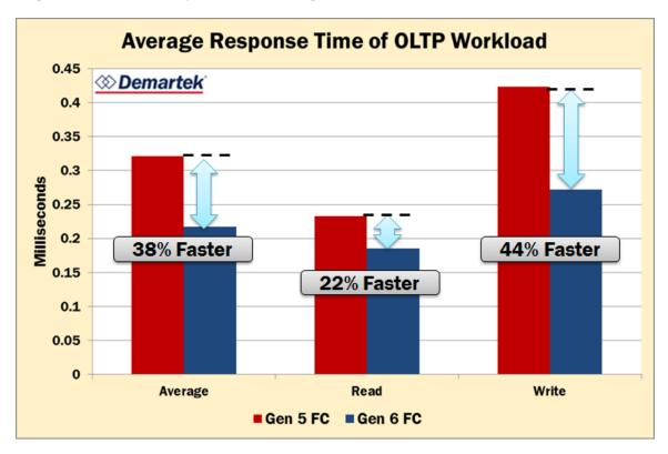
The workload never reached Gen 5 FC limits for bandwidth or IOPS, so neither the HBA nor switch was saturated by I/O requests. The response time improvements can be attributed strictly to the upgrade from Gen 5 FC to Gen 6 FC. Latency was sub-millisecond in all cases, but the deployment of Gen 6 FC was responsible for
