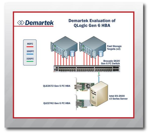
A private SAN was implemented for this evaluation, with Gen 6 FC technology only deployed at the host and Brocade G620 Gen 6 FC switch. High-speed storage targets hosted database and replication volumes with a combined 14 lanes of 8 Gbps FC<sup>3</sup>.
