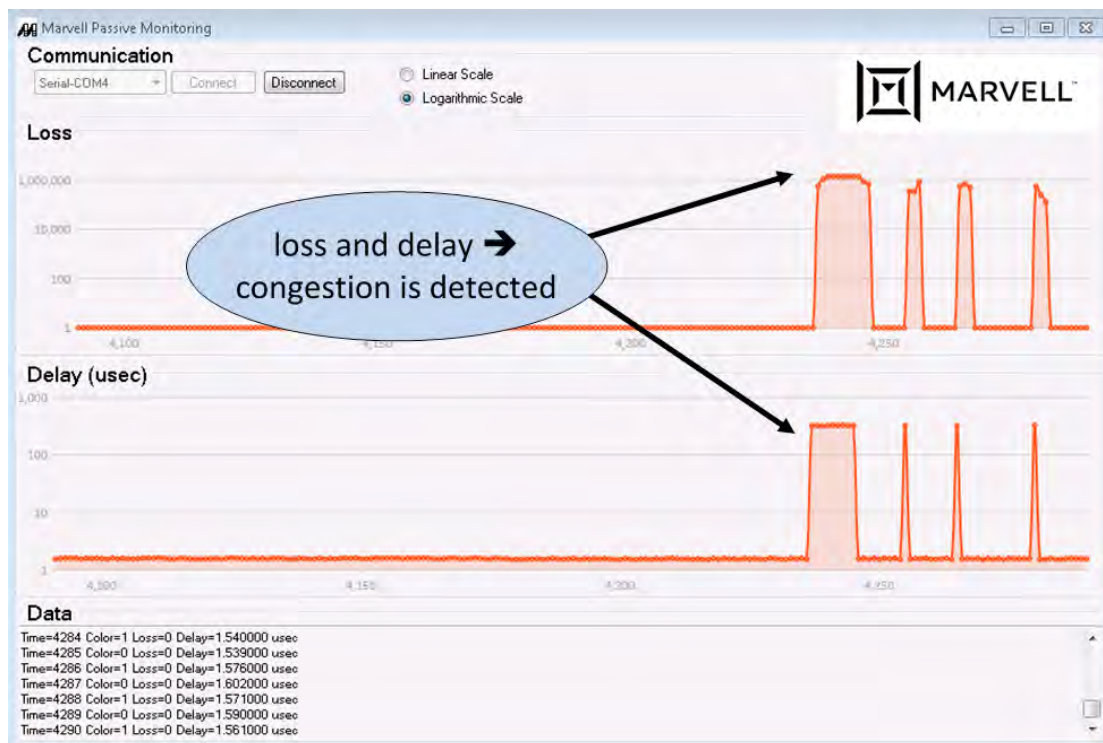
Figure 8: Loss and delay measurement using alternate marking. The horizontal axis represents time (seconds), and the vertical axis represents the delay in microseconds (bottom graph), and the number of packets lost per second (top graph).
