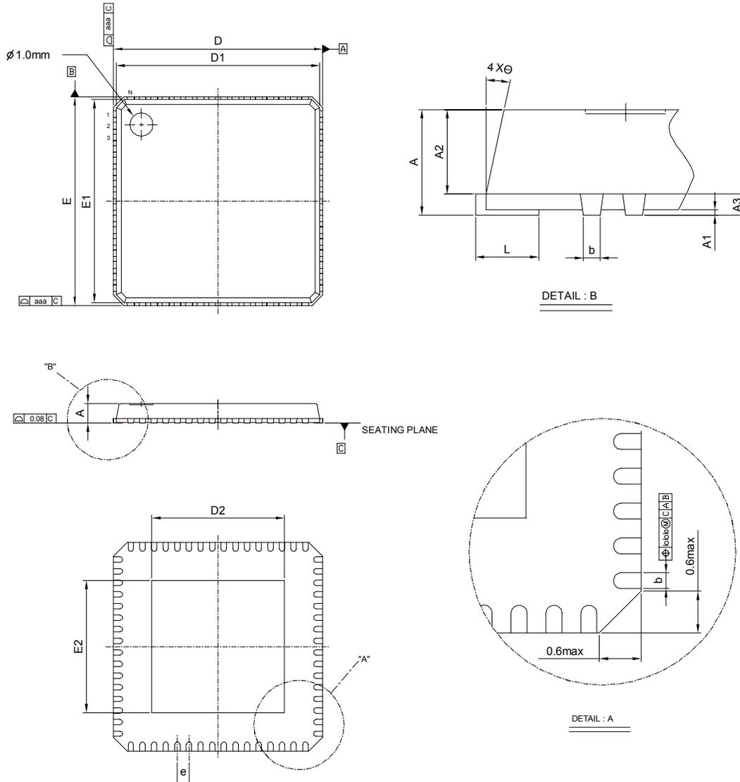
**Table 10: 64-Pin QFN Mechanical Dimensions**
